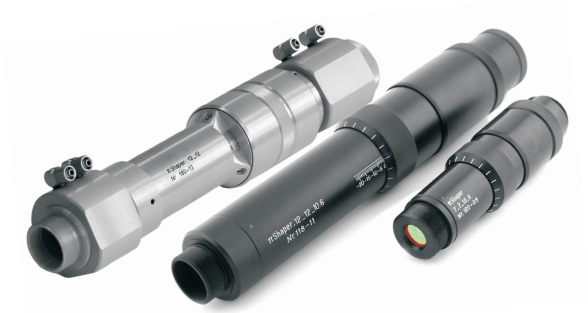
With these unique tools it is possible to convert a single mode or multimode laser beam of similar to Gaussian intensity profile into a collimated Flattop beam with nearly 100% efficiency.
